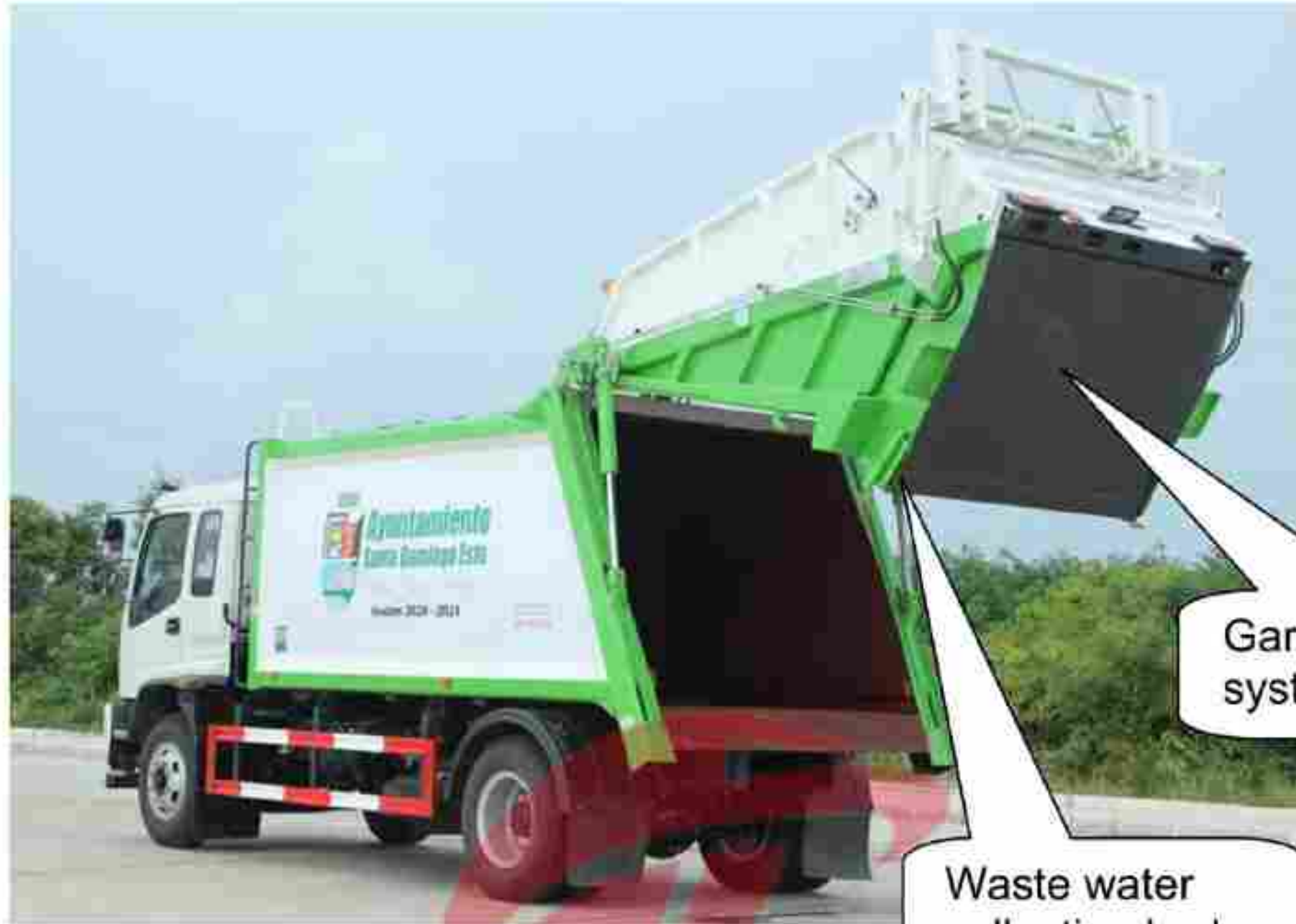
Front View: garbage collection system and waste water collecting bins
