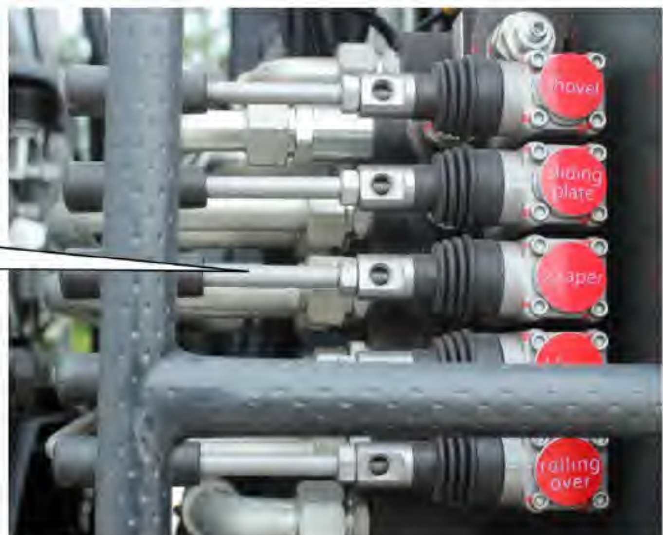
Hydraulic Control Joysticks (At drive side)
