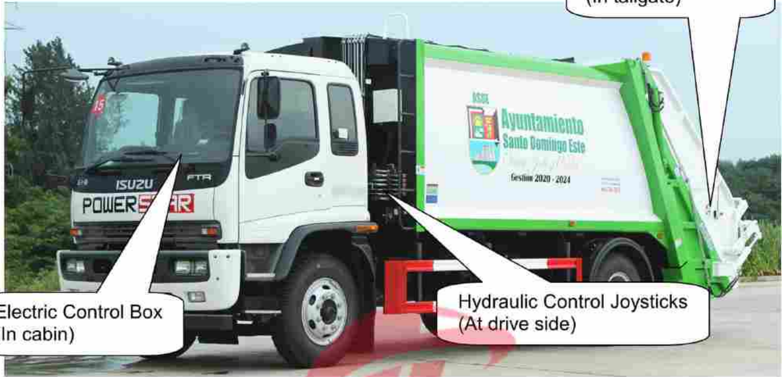
Front View: Hydraulic control system
